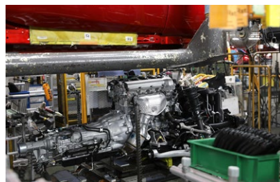
The domestic Skyactiv-G 1.5-liter engine being built. The engine is produced in a separate factory at the same time as the body, with the pair later mated on the line.
